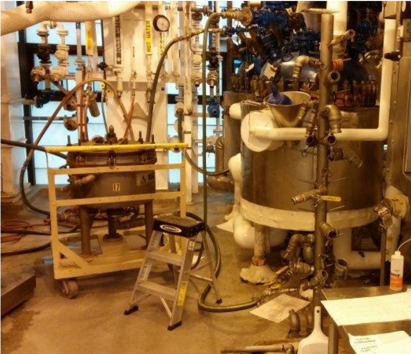
A 400 liter reactor in the process of converting shavings of corn stover.(Photo: Mercurius Biorefining)
